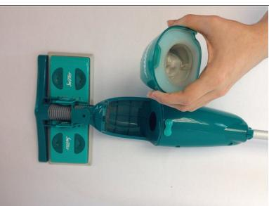
Lift the dirt container out of the device housing.
