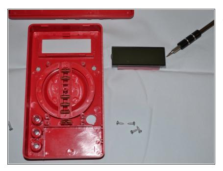
• Carefully remove screen from device by lifting upward.
