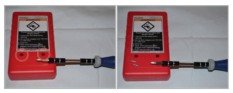
Unscrew the two 9mm screws on the back panel using a #0 Phillips screwdriver.
