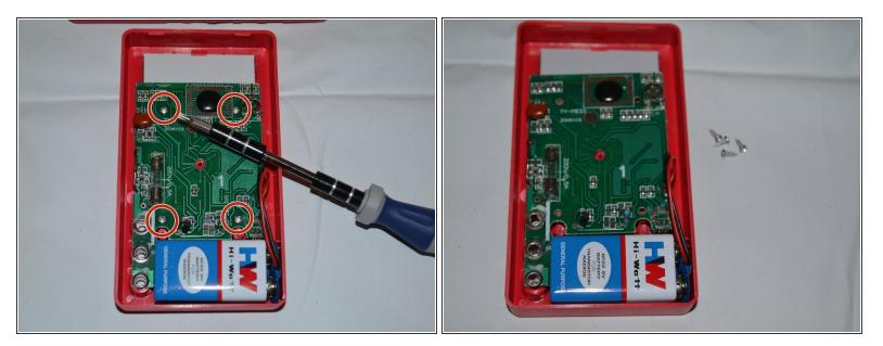
• Remove the four 7mm Phillips screws holding the circuit board in place.
