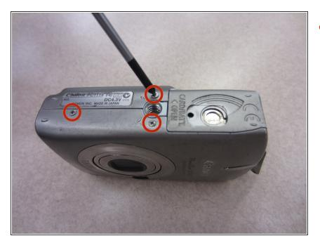
Remove three .15 inch Phillips screws from the bottom of the camera using a #00 Phillips screwdriver.
