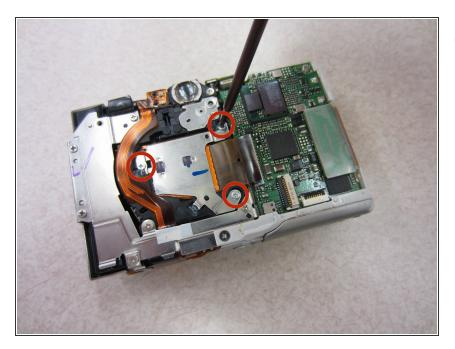
Unscrew three .15 inch Phillips screws from the back of the camera using a #00 Phillips screwdriver.
