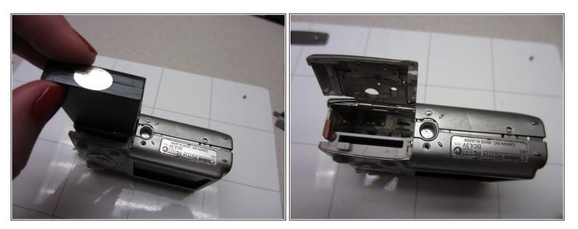
Slide the battery out of the battery compartment.
