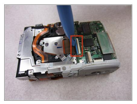
Place the pry tool under ribbon gate and gently lift it up, disconnecting the ribbon.
