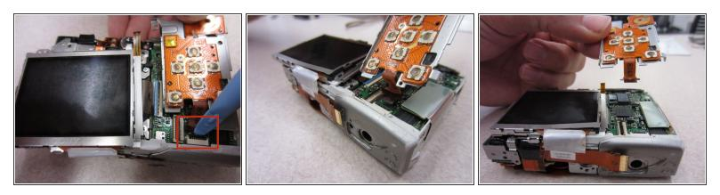
• Remove the ribbon with a pry tool by gently pulling it out of the ribbon gate tab.
