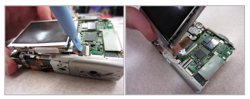
Gently press the pry tool under the ribbon gate and lift up to free the ribbon connecting the LCD to the circuit board.
