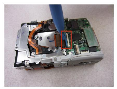
Place the pry tool under ribbon gate and gently lift it up, disconnecting the ribbon.
