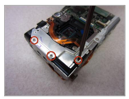
Unscrew three .065 inch Phillips screws using a #00 Phillips screwdriver from the back of the camera.
