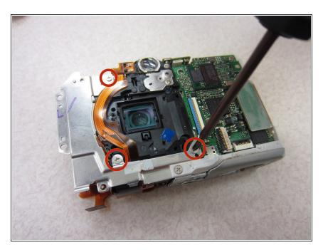
Unscrew three .12 inch long Phillips screws using a #00 Phillips screwdriver from the back of the camera.
