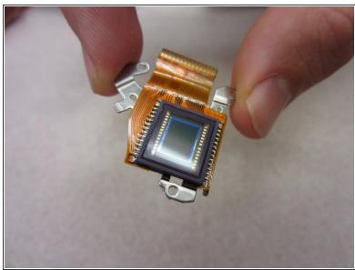
Use the pry tool to gently lift the image sensor away from the rest of the camera.
