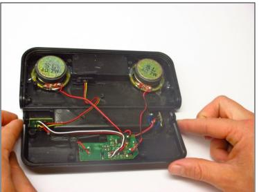
• Remove the back cover carefully; there are many wires that connect it to the device.
