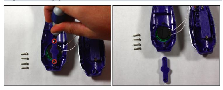
• Remove the 2, #8 11.7 mm speaker guard screws with the Phillips Head screw driver.
