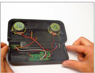
Remove the back cover carefully; there are many wires that connect it to the device.
