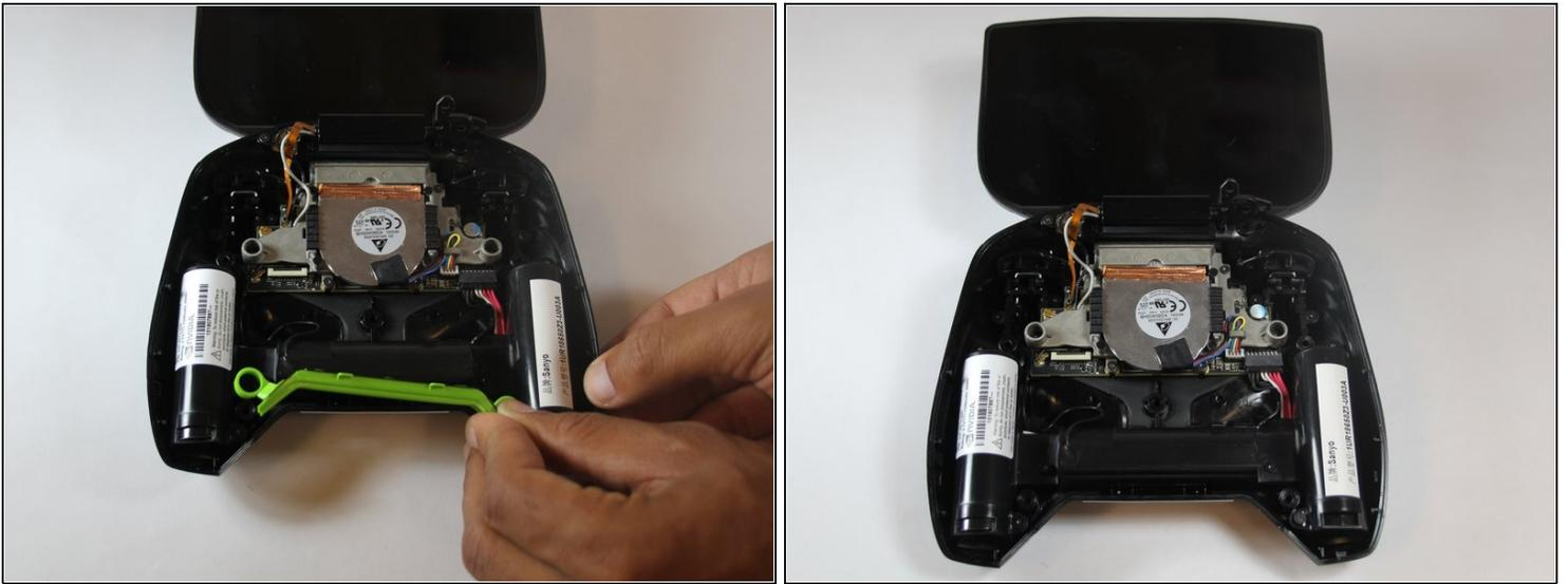
**i** The green grill is not screwed in so it can be pulled right out.
