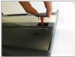
The Power button can now be removed/clean/replaced.
