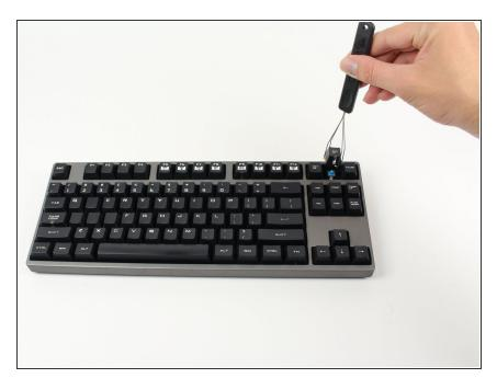
Pull cap directly upward.
