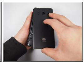
Remove the rear cover on the back by pulling up on the gap located at the bottom of the phone.
