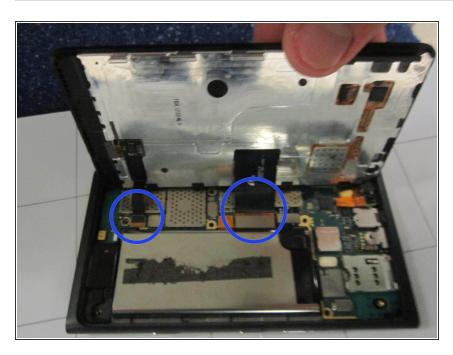
Detach both ribbon connectors from the logic board.
