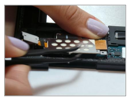
After all the screws have been removed lift the circuit board up to wiggle free.
