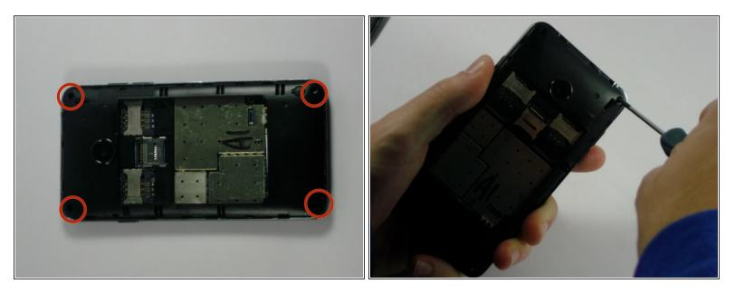
Use a screwdriver to remove each of the four screws.
