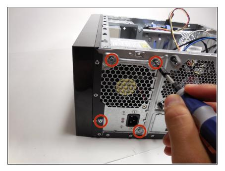
Using the Phillips #2 driver, unscrew the four 8mm screws attaching the power supply unit to the outside of the computer.
