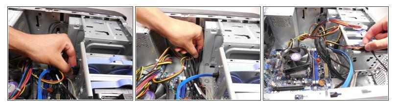
• Unplug all cords attached to the optical drive and hard drive.
