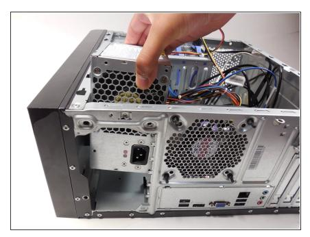
• Remove the power supply unit by pulling away from the screw side and then out.
