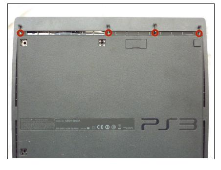
Remove the four 13.3 mm T8 security Torx screws beneath the Blu-ray drive opening. (Some models may only have three screws)
