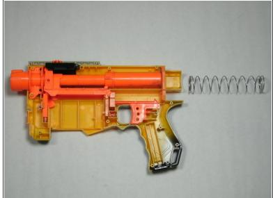
Pull the spring out the back of the gun.
