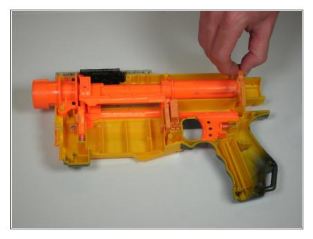
Lift the plunger guide straight up out of the gun.
