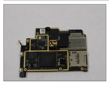
After removing all screws and disconnecting all cables, the board should easily lift up off of the device housing.
