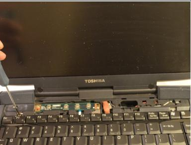
Unscrew the two screws near the top of the keyboard.
