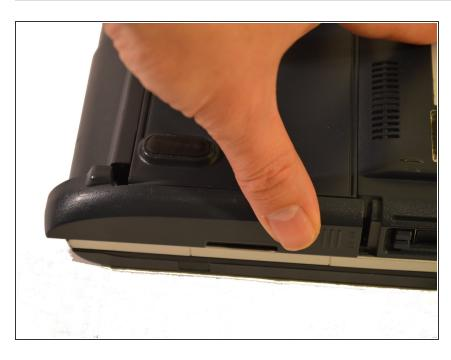
With one finger on the raised grip, slide the latch towards the front of the laptop.
