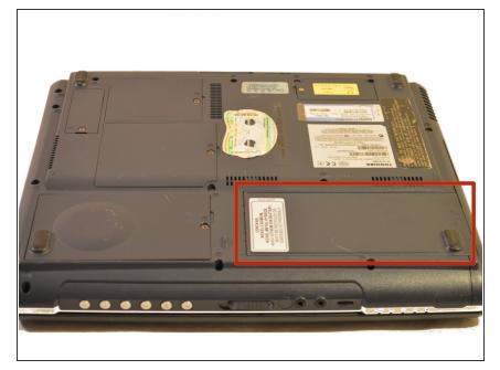
The battery is located on the front right corner of the laptop.
