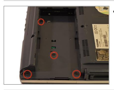
Unscrew the screws located beneath the battery.
