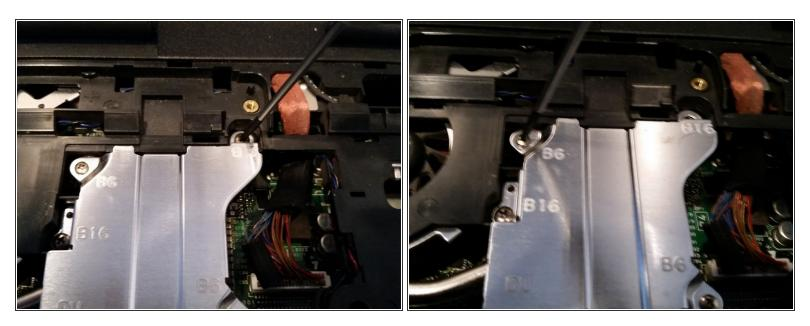
Unscrew all visible screws on the heat sink shield.
