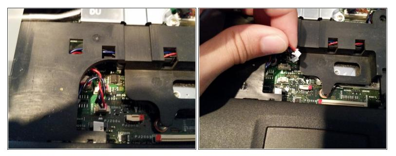
• Disconnect both speaker connectors located near the center of the laptop.
