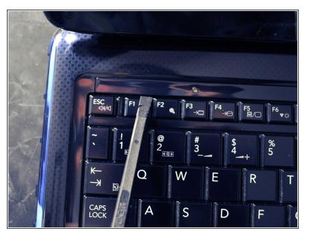
• Use a spudger to carefully pry up the keyboard screw cover.
