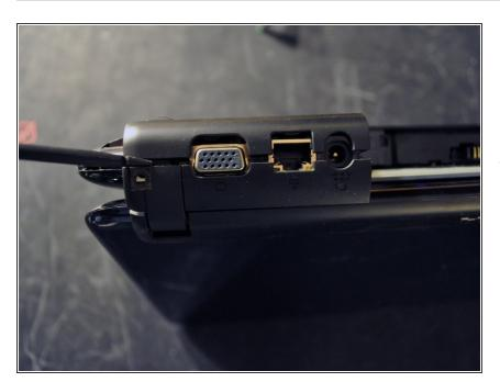
Carefully work a spudger in the crack at the back of the laptop and separate the small rubberized
