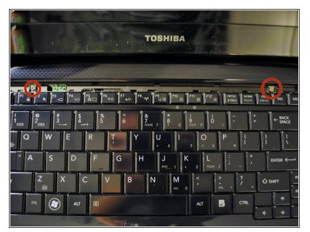
• Remove the two screws securing the keyboard to the chassis.
