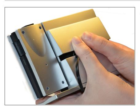
To remove the battery compartment cover, slide the cover up towards the top of the clock while applying slight pressure.
