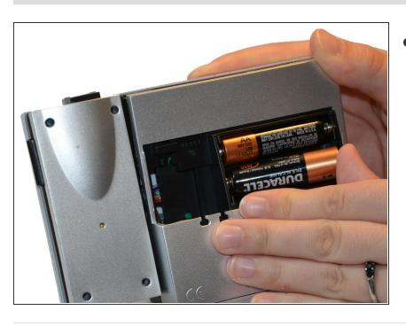
Once the old batteries are removed, insert new AA batteries.
