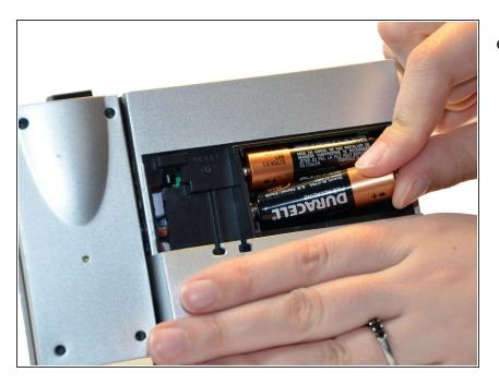
Using your fingertips and lifting up, take out the two AA batteries.
