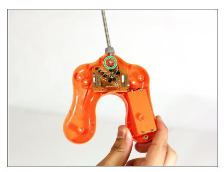
Remove the 7.9 Phillips #1 screw that holds both the antenna and the internal chip.
