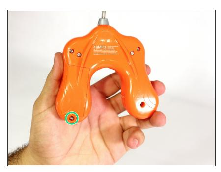
The battery cover 8.0mm Phillips #2 screw is on the bottom left handle.
