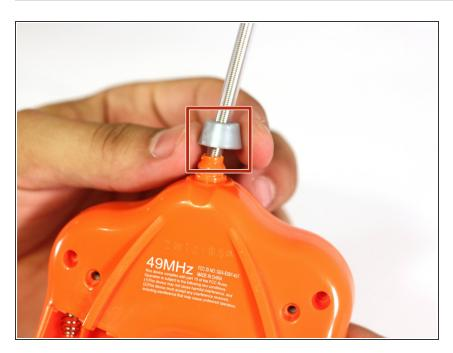
Lift the antenna holder away from the controller towards the top of the antenna.
