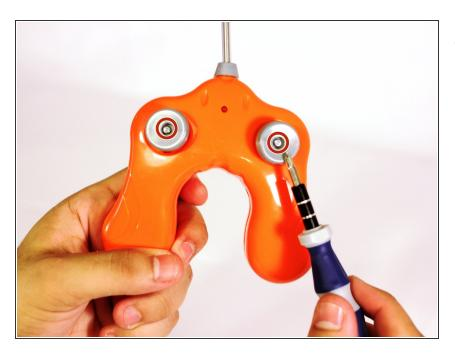
Remove both 6.0mm Phillips #1 screws holding the D-pads in place.
