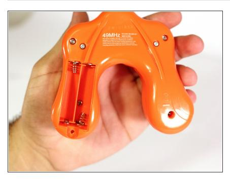
Remove the 2 AA batteries.
