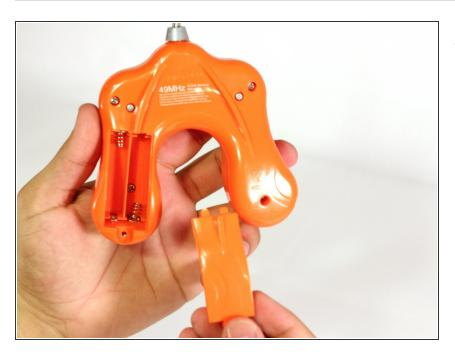
Once the screw is removed lift the battery cover up from the controller.
