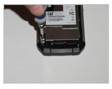
Next, remove the two torx (starshaped) screws below the battery. These screws help to secure the outer shell of the phone around the motherboard. A T-5 bit is required for removal.
