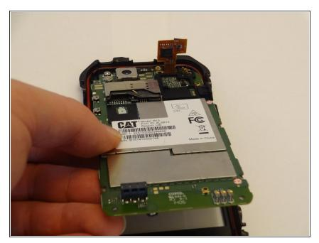
Finally, disconnect the chip seen in the upper right, and the board should pull away from the rest of the phone.
