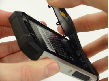
Remove the back covering by gently lifting upwards from the bottom of the back covering. The back will snap off and the battery is exposed.
