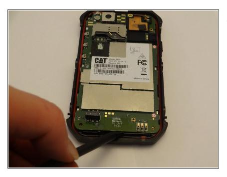
With all screws removed, move around the motherboard, carefully prying it from the remaining shell.
