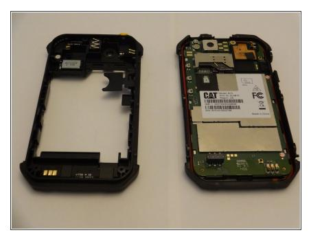
With all screws removed, the back and side pieces should come off the front of the phone, exposing the motherboard and various components as shown.
