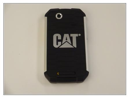
Place the phone screen-side down and place thumb on the yellow and black switch. Slide the switch to the right to unlock the back covering for removal.
