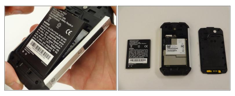
Place index finger at the top edge of the battery and gently lift upwards. The battery will slide cleanly out of the phone.
