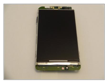
Installing the new LCD is the reverse of removing the old one. The 2mm 3M adhesive tape listed in the guide is recommended for fixing the new display to the board.
