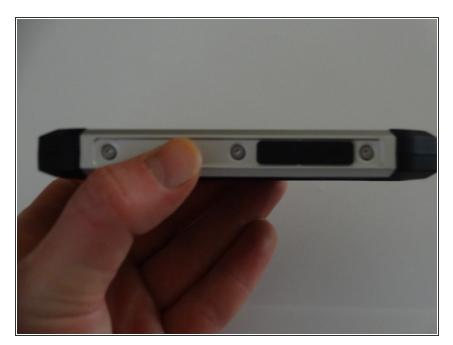
There are three remaining screws on each long side of the phone. A small hex bit is required for removal.
