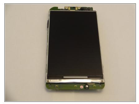
With the device completely disassembled, the LCD can easily be accessed. It is pictured here, in which it adheres to the front of the motherboard.
