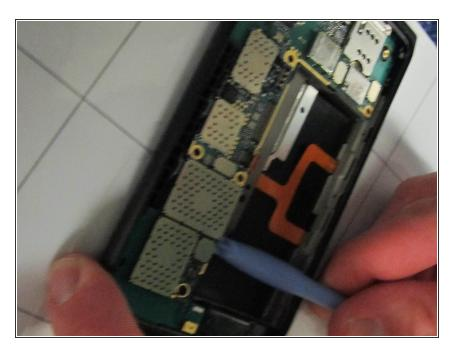
Using a pair of tweezers, remove rubber gaskets that are holding the motherboard in place.
