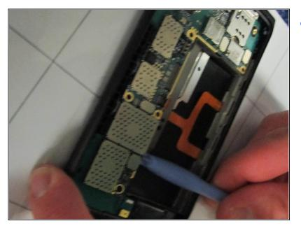
Using a pair of <u>tweezers</u>, remove rubber gaskets that are holding the motherboard in place.
