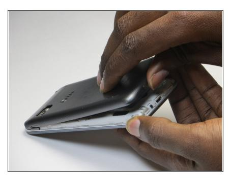
Remove the back device of the LG VM720.
