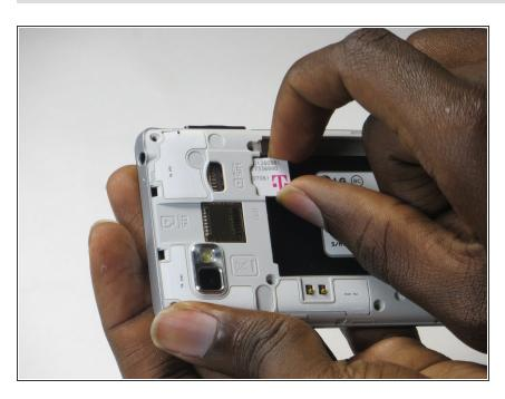
Use the fingertip cutout to help push the old sim card out. The sim card should exit toward the direction of the battery
