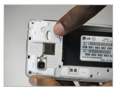
When the back cover is completely removed, locate the sim card slot. It should be right above the the battery and it is clearly labeled "Micro Sim"
