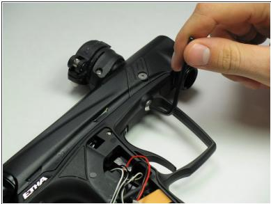
• Use the 1/8" hex key to remove the two dome-headed screws by rotating them counter-clockwise.
