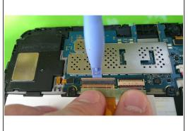
Once all 10 screws have been loosened and removed, you can now use your plastic tool to lift up one edge of the battery. Disconnect the wire from the motherboard by pressing on the small white latch where the wire connects. Remove the other wires on the device in the same manner. Once the wires are removed it is safe to remove the battery.
