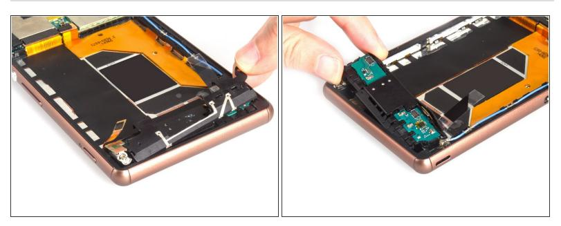
Remove loudspeaker assembly cover and assembly itself.
