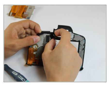
Remove the speaker by firmly gripping the top of the speaker and pulling down towards the bottom of the back panel while rotating the top of the speaker upwards, away from the back panel. This will allow the speaker to come off of its pivot point.
