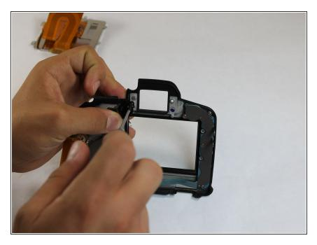
Remove the single 4.8 mm screw using a Phillips #0.
