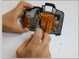
Remove each of the 3.4 mm screws holding in the LCD using a Phillips #0.
