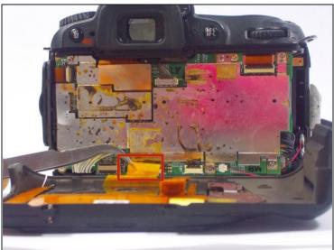
• After, remove the two orange ribbon connectors attached to the interior of the camera with <u>tweezers</u>.
