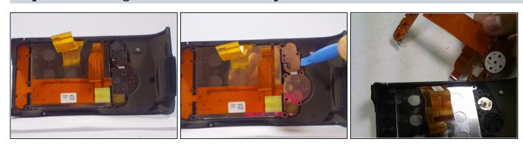
Use a plastic opening tool to separate the LCD and metal plates from the casing.
