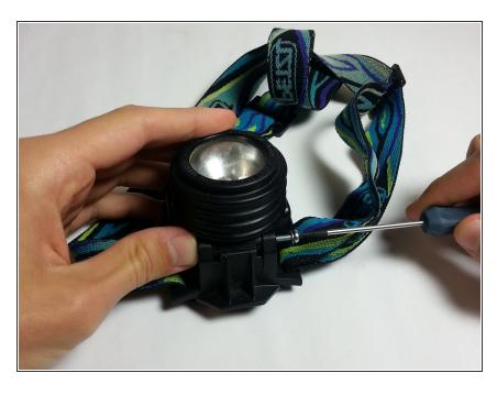
Tighten the new bolt into the new nut by turning the bolt clockwise using a Phillips head screwdriver until the bolt & nut are tight.
