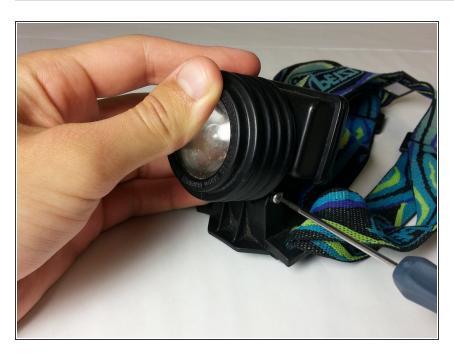
Remove the old nut and bolt by using a Phillips head screwdriver to rotate the bolt counterclockwise until it becomes free. The nut should become free on its own as the bolt is removed. If it doesn't, poke the nut out using the screwdriver.
