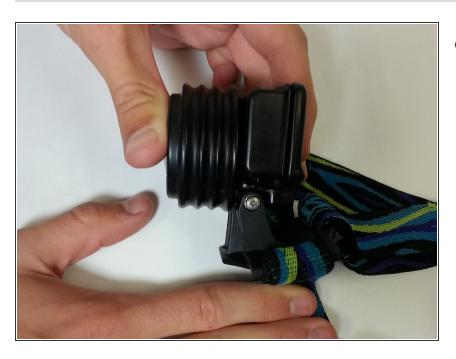
Check the mount assembly for a loose or missing nut and/or bolt.
