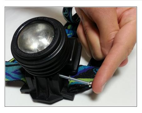
Insert the threaded portion of the new bolt with the washer into the right side of the circular hole created
