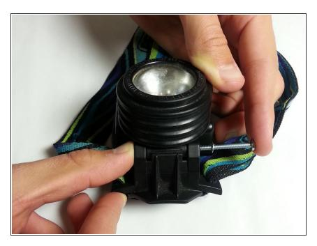
Firmly hold the nut in place with your left thumb such that the nut will not rotate.
