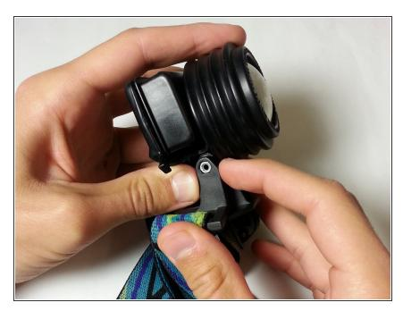
Insert the new nut by placing it in the left side of the circular hole created after the removal of the old nut & bolt in step 2.
