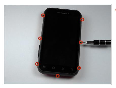
Using the screwdriver and the T-5 bit, unscrew the seven 5 mm screws around the outside of the phone.
