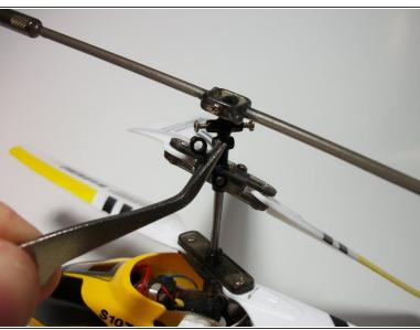
Using tweezers, gently remove the two stabilizing links by pulling straight away from the point of connection.
