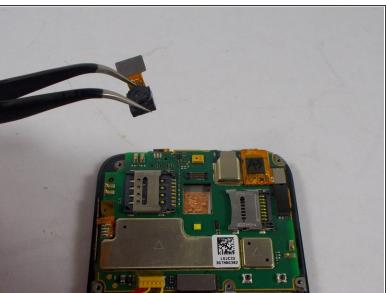
Use a pair of tweezers to gently disconnect the camera connector and remove the rear facing camera.
