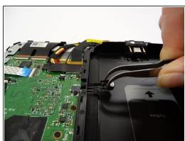
With tweezers gently squeeze and remove docking indicator device
