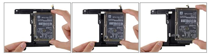
• Lift the hard drive up and remove it from the drive tray.
