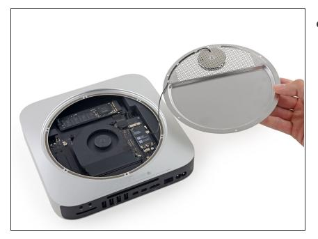
Remove the antenna plate from the Mac mini.
