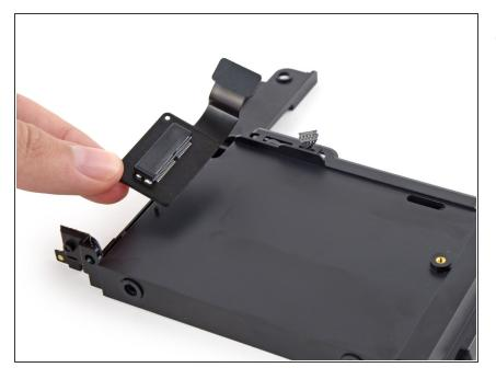
• Remove the PCIe SSD cable from the drive tray.
