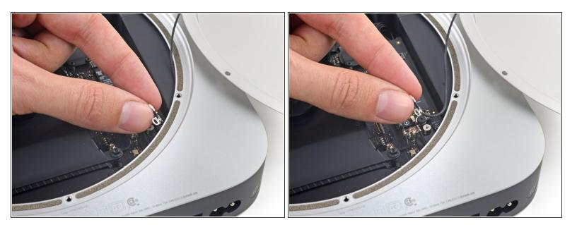
• Carefully pull the antenna cable out from the gap between the power supply and case.
