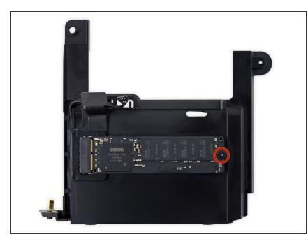
• Remove the 5 mm T5 Torx screw securing the SSD.
