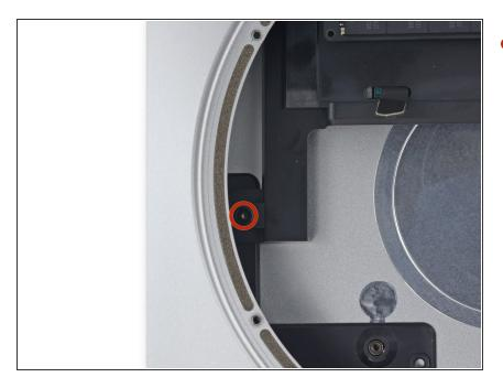
Remove the single 8 mm T6 screw securing the drive tray.
