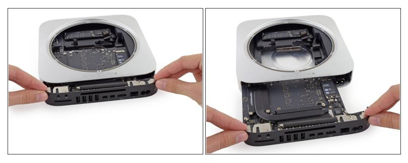
Carefully slide the logic board assembly out of the Mac mini, minding any cables that may get caught.
