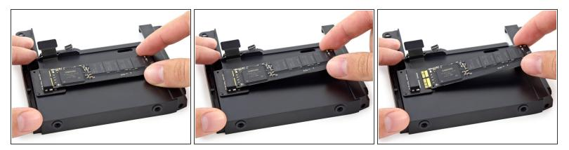
• Lift the free end of the SSD up slightly and pull it out of its socket.
