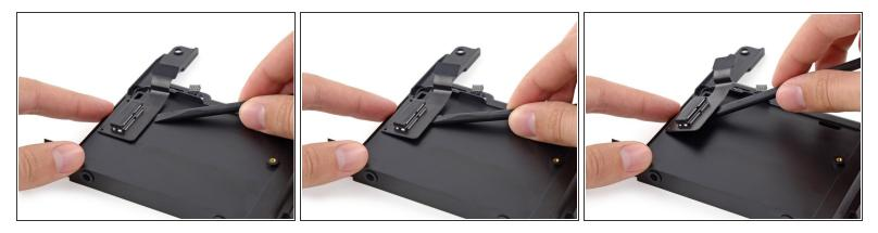
• Slip the flat end of a spudger under the SSD cable to lift it off the adhesive holding it to the drive tray.
