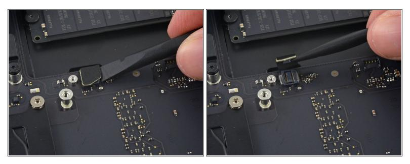
Use the flat end of a spudger to lift the SATA cable connector up off of its socket on the logic board.
