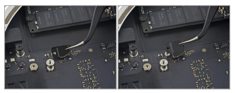
• Remove the SATA cable connector bracket.
