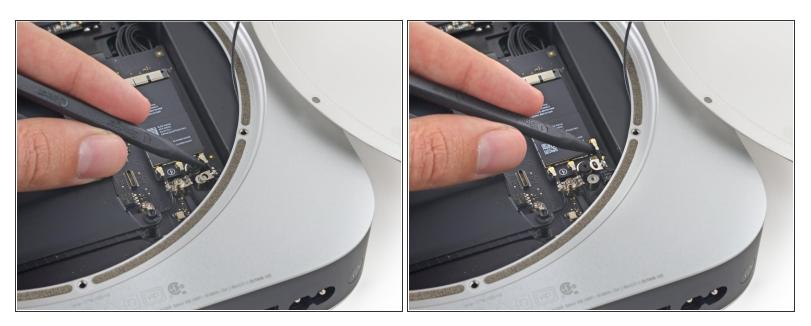
• Use the point of a spudger to lift the antenna connector straight up off its socket on the airport card.
