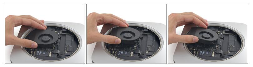
(i) The fan connector is trapped under the edge of the fan and cannot be disconnected until the fan is moved.
