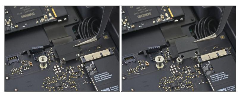
• Remove the PCIe SSD cable bracket.
