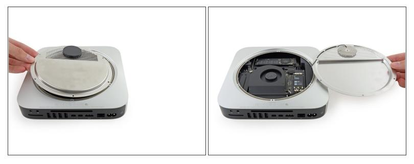
▲ Do not completely remove the antenna plate; it is still connected to the Mac mini by an antenna cable.
