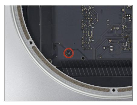
• Remove the single 16 mm T6 screw securing the logic board.
