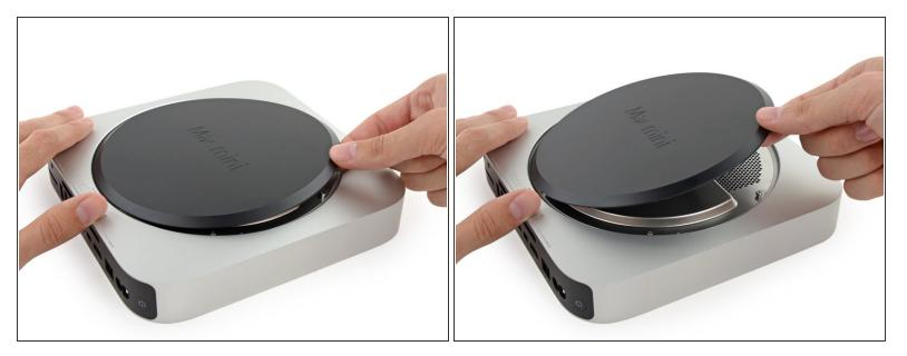
• Lift and remove the bottom cover.
