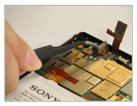
Use the tweezer, carefully pry open the chip for the back facing camera.
