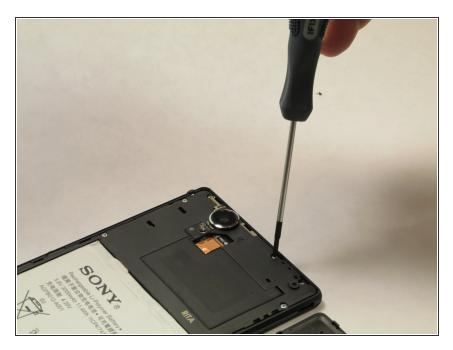
Using the Phillips #00 Precision screwdriver, take out 8 silver screws (3.15mm) and 5 gold screws (3.9mm) for a total of all the screws attached to the flat plate. 3 of the gold screws are located at the top of the phone and the other 2 screws are located at the bottom of the phone.
