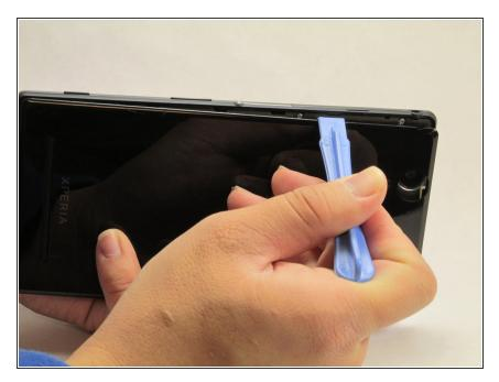
Using the spudger, pry open the back cover by starting alongside the edge of the back cover.
