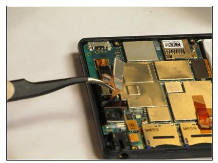
To take out the back facing camera, flip open the flap labelled 'film' to reveal the chip that connects to the motherboard.
