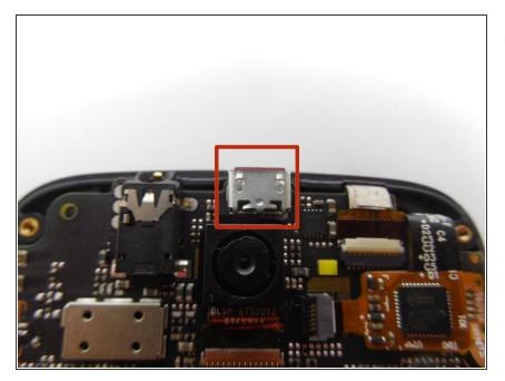
Once the old charger port is removed, take the new one and place it in the same spot. You will need to solder this piece to ensure that it stays connected.
