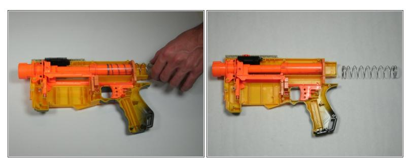
• Pull the spring out the back of the gun.
