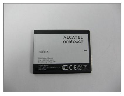
This is the battery for the Alcatel One Touch Evolve. Look for this component when the back panel has been removed.
