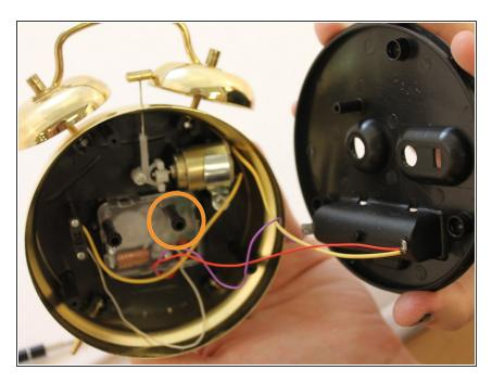
After removing the three screws on the back cover you can work inside the clock to fix the alarm knob.
