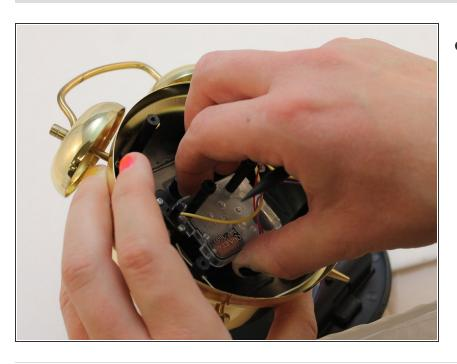
Because the alarm knob is attached to the wiring box you need to remove the whole box to replace the knob with a new one
