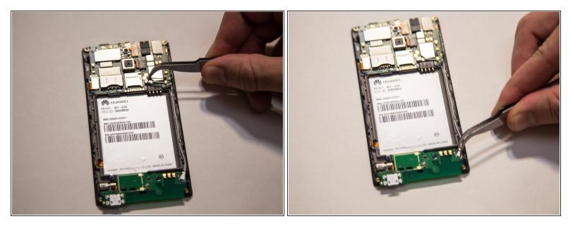
• Lift gently at each connector of the white wire to disconnect the antenna from the port.
