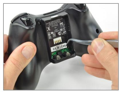
• Use a pair of tweezers to peel the barcode sticker from the battery compartment.
