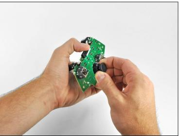
• Remove the left analog stick cover using the same procedure previously described.
