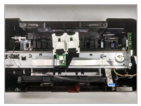
• Pull the belt tightly to this side, creating enough slack to lift the belt from the wheel.
