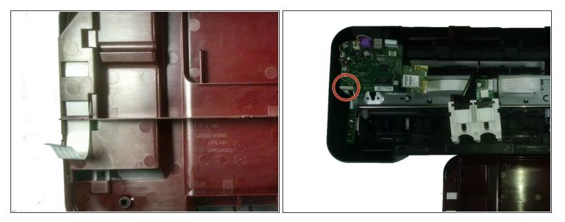
• Detach the wire from the printer by pulling the blue-sealed end from the white holder.
