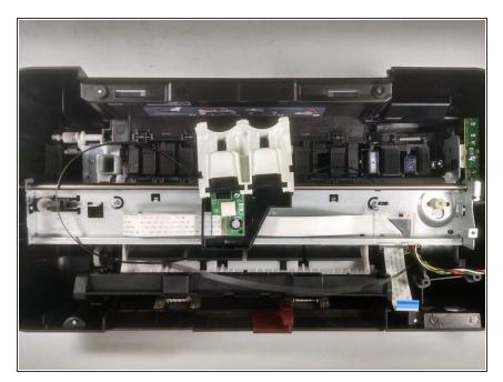
• Lift the metal structure from the printer, which will include the ink cartridge holders.
