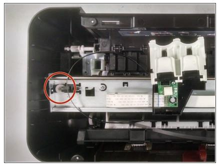
• Locate the belt, and the wheel it is around. The wheel will be on top of the metal piece on the far right side.
