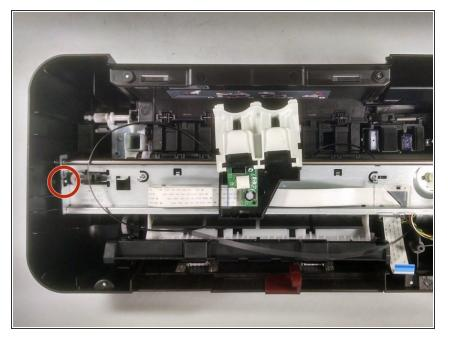
On the left side, between the wall of the printer and the metal piece, there will be a spring connecting the two. Use the tweezers to detach the spring and keep separate.
