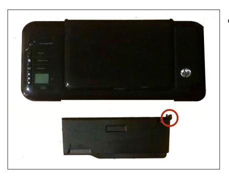
• To release the tray from the printer, you must manually pull it out. Hold the tray and push towards one side of the printer. Then pull away from the printer towards the other side. Keep output tray separate.
