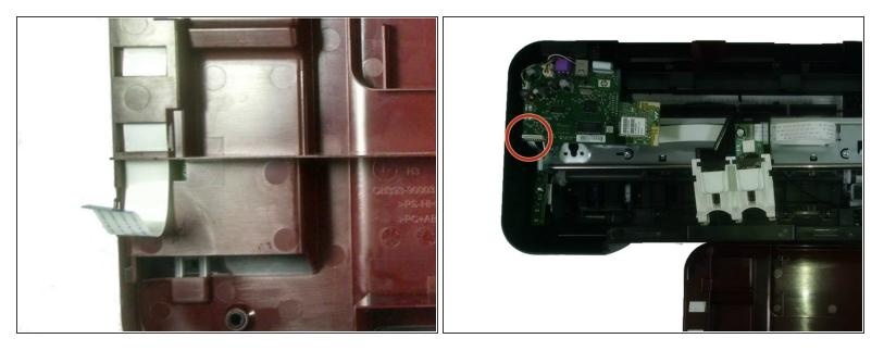
• Once the top is loose, there will still be a connection wire between the printer and the cover. This wire will be about one inch wide and white, located under the buttons.
