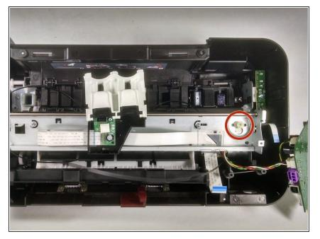
Push the ink cartridge to the center of the printer so that the wheel on the opposite side is visible. Then lift the belt from that wheel.
