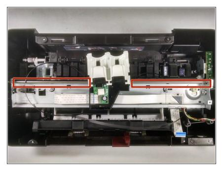
Locate the metal bar that will be running parallel to the metal structure that was just removed.
