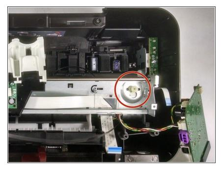
• Remove the metal bar that the motor is attached to.
