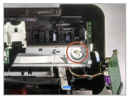
Now releasing the metal structure will be possible. On the left side of the structure, locate the wheel that the Carriage Driver Belt was around. Push this wheel through the larger opening it sits in.
