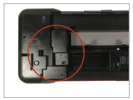
• Flip the printer upside down and locate the cover on the left hand side. It is rectangular shape and is
