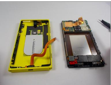
Once the metal clip is removed, gently pry up on the ribbon cable connection, located underneath the metal clip you have just removed.
