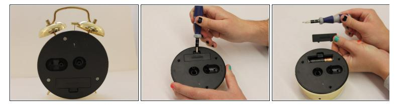
• Remove the battery door using your finger nail or an opening tool.
